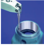
GT 31 with lever in perpendicular position
