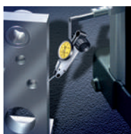
Perpendicularity using TESAST
