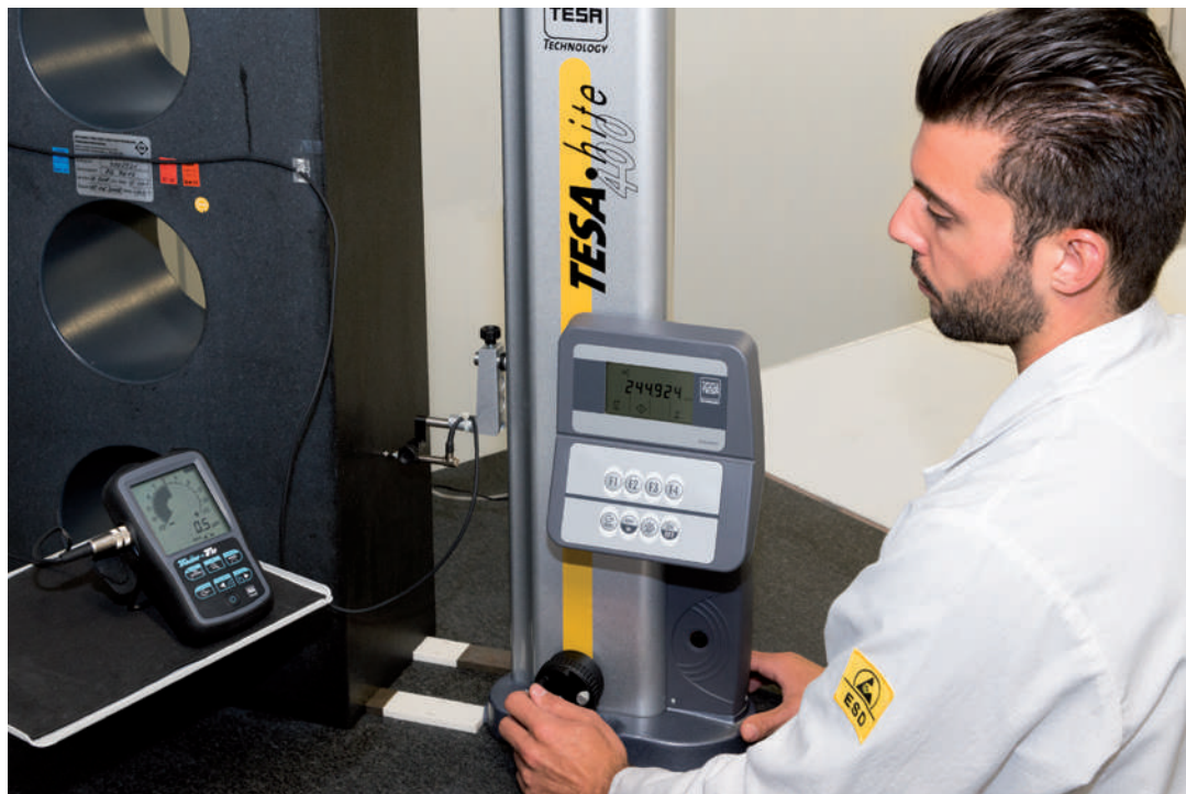
Squareness verification with inductive probe and TWIN-T10 display
